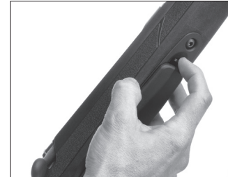
Press the magazine release rearward. The magazine will fall into your hand.
