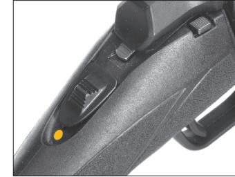
"Safety" shown in the off safe position.
