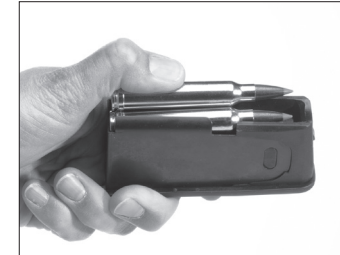
Press the cartridge straight down until it snaps into place under the feed lips.
