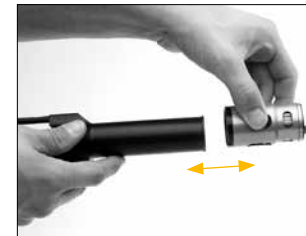
Separate the gas system components to simplify cleaning.
