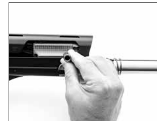
Pull outward to remove the bolt handle.
