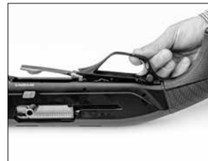
Lift the trigger group from the receiver.
