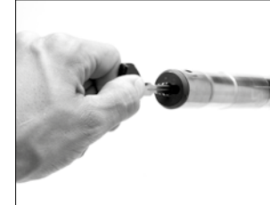
Use a key or small screwdriver to press in on the three-shot adaptor, then rotate a quarter-turn.
