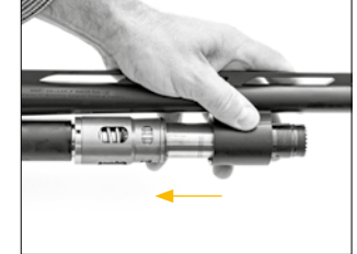
Slide the barrel and piston over the magazine tube and the barrel extension into the receiver.
