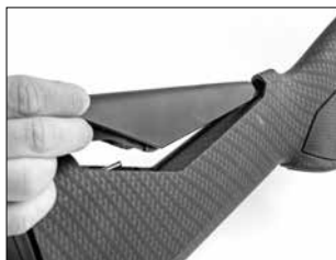
Insert the front of the cheek piece into the stock housing and lower the rear section to install. Tighten the rear screw, being careful not to overtighten.
